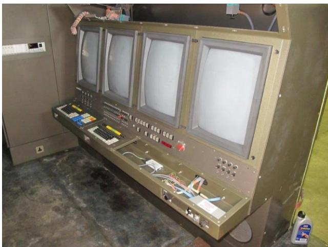
**Display Console with missing top switch panel and Engagement Controller's keyboard**
