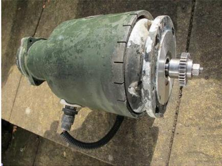
**T86 Elevation Motor after Removal and Cleaning**
