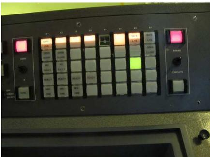
Missile 7, green 'No Fault' It should not be on!
