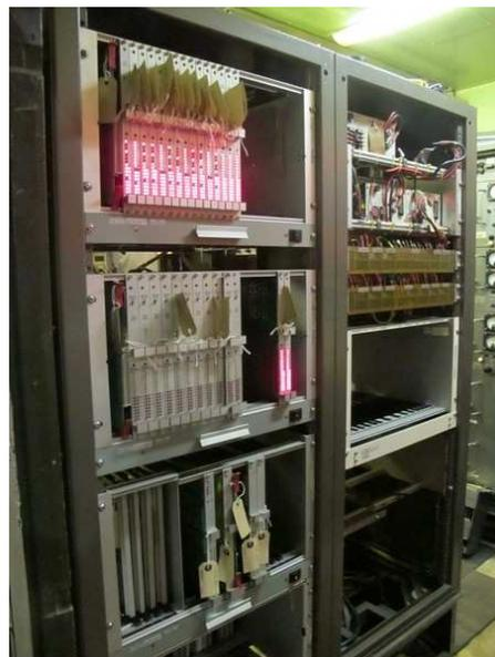
Power Supplies for the Digital Input and Output Chassis Reinstated
